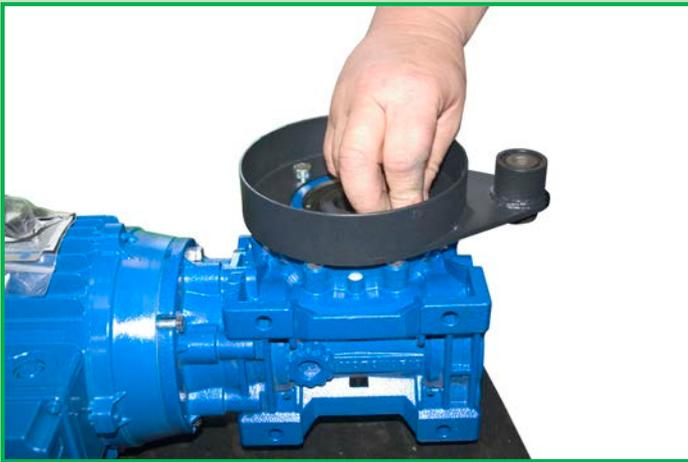
Press fit the torque arm bush into the torque arm; then fasten the torque arm to the GMU with the shaft sleeve facing away from the gearbox before attempting to fit it onto the drive shaft.
