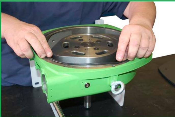
The O-ring should sit securely in the groove located around the front of the pump housing. A small amount of grease may be required to hold the O-ring in place. The front cover should bolt in place with the use of cap head screws and washers.
