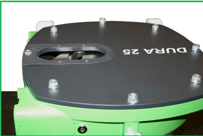
Fit the inspection window gasket to the front cover.
