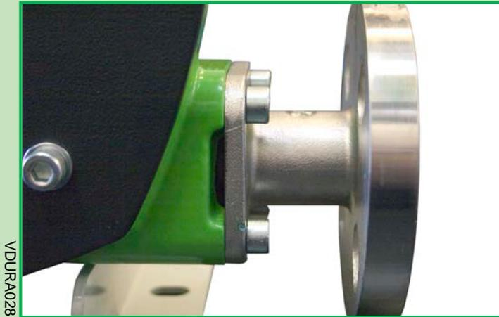
The tapered flange should be pulled toward the housing for as close as is possible ensuring 5mm (16") of the hose can be seen in the gap between the fixing holes.
