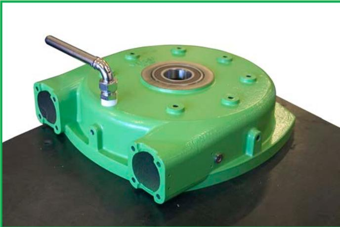
It is also important at this point to attach the filler tube to the back of the pump as it could be difficult to attach once the Geared Motor Unit (GMU) is in place. Line the thread of the breather tube with PTFE tape and tighten into position to give a leak free seal.
