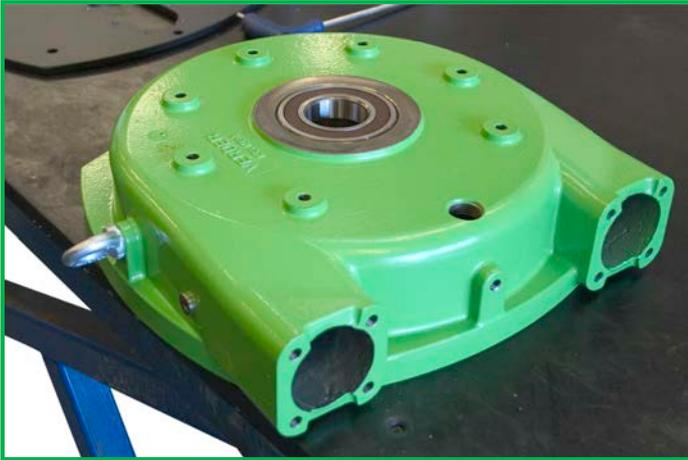
Fit the lifting eye to the case.
