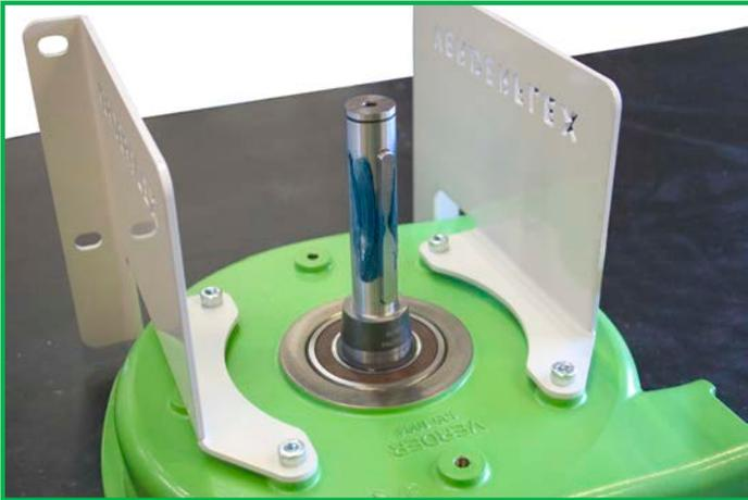
Grease the shaft before fitting the GMU.
