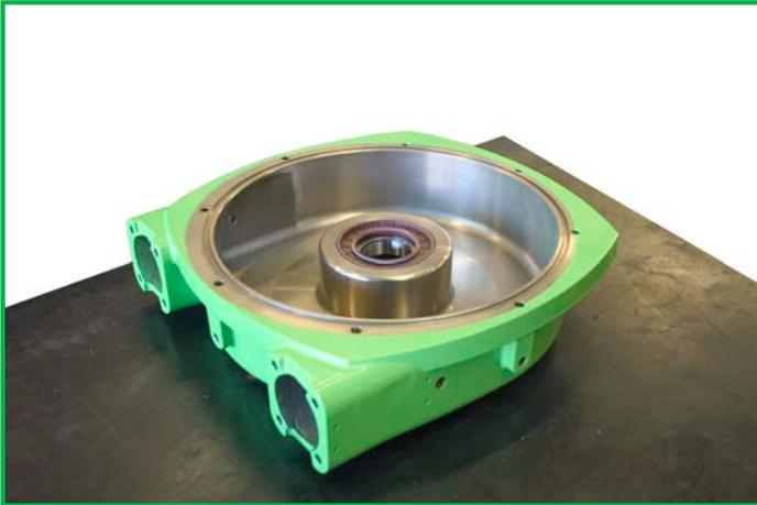
The shaft seal should be pressed squarely on top of the inner bearing with the sprung lip facing into the pump cavity.
