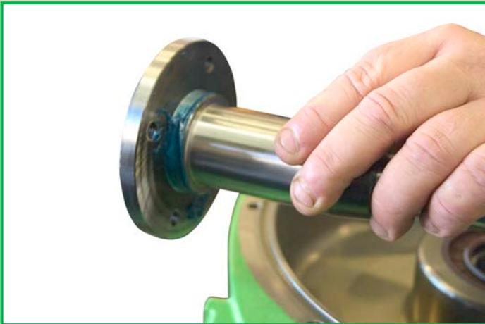
Apply some triple life bearing grease (Rocol Sapphire 2) to the drive shaft before assembly.
