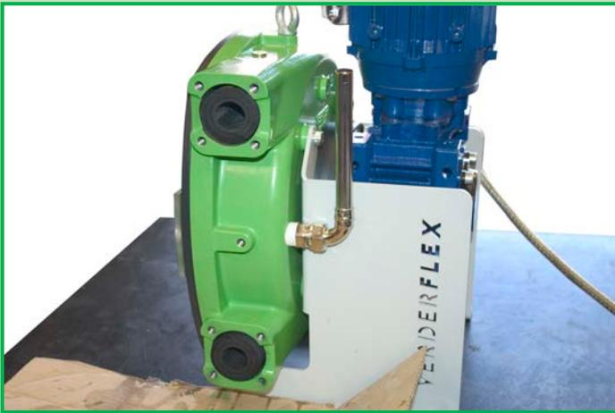
The hose should be inched forward until there is sufficient hose protruding from the suction and discharge ports to fit the tapered flanges (10mm). If the hose passes this point the drive should be reversed and inched back slowly into the correct position.
