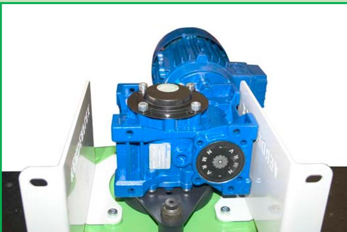
To complete the assembly, mount the dust cover using the screw cap head screws supplied.
