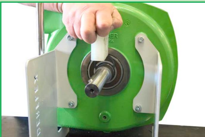
Once the drive shaft is in place the crescent ring groove should become visible at the rear of the pump. It is recommended to lock the drive shaft in place with the crescent ring before bolting the rotor in place.
