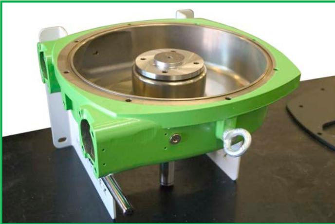
Press the drive shaft through the bearing assembly.
