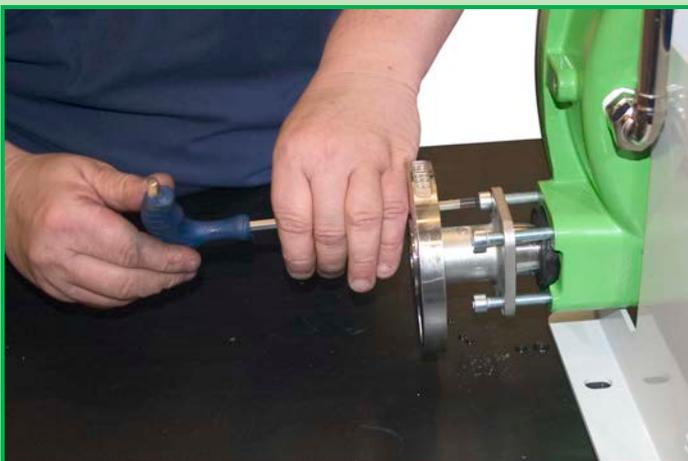
Tightening the bolts in a 1-3-4-2 sequence, repeating the sequence until the flange is evenly fitted. All 4 bolts should be fitted to each flange to avoid compromising the performance of the pump.
