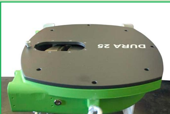
When fitting the front cover, the cap head screw nearest to the inspection window, is fitted without a washer (pictured).
