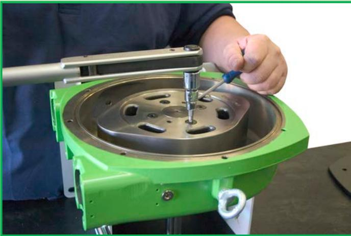
Secure the rotor to the drive shaft using 4 countersunk socket cap head screws. Failure to use all of the screws could compromise the performance of the pump.
